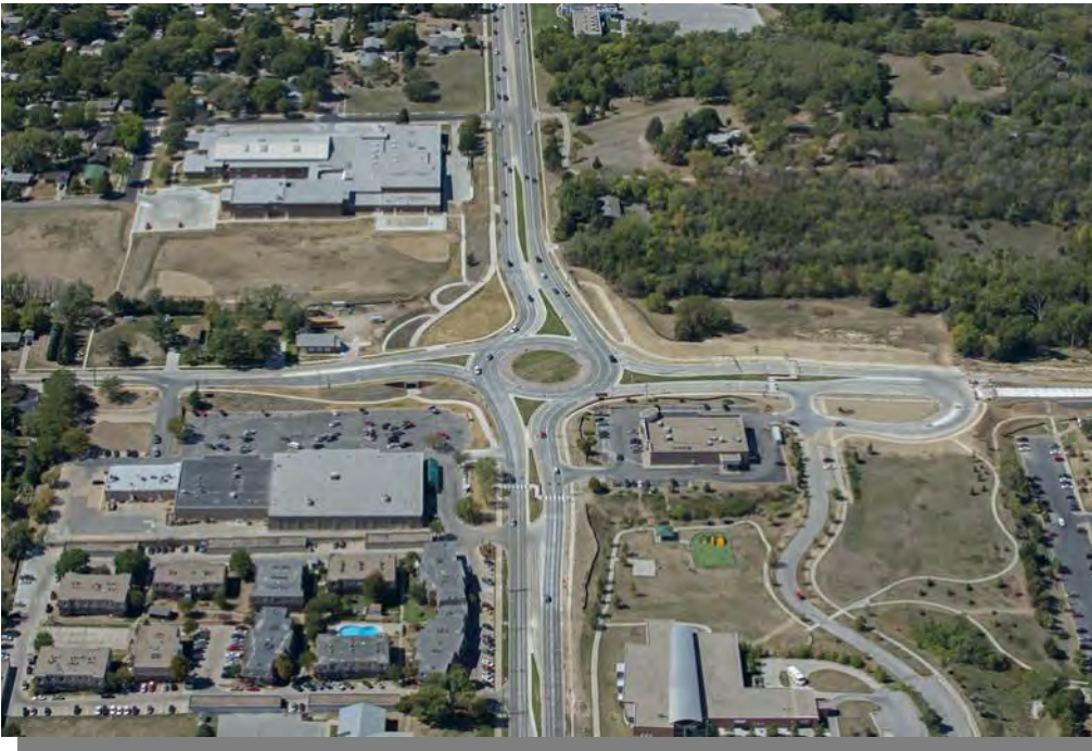
Figure 6.7: Example of a Three-lane Roundabout
